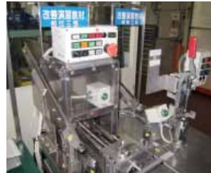
Assembly attachment and inspection practice education materials. These integrate various defects and if the proper improvements are made, work time can be shortened from 19.6 seconds to 6.3 seconds.
