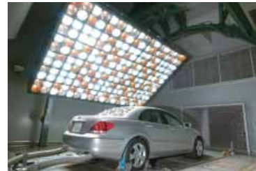
Environmental resistance testing (Reliability Center of DENSO Corporation)
