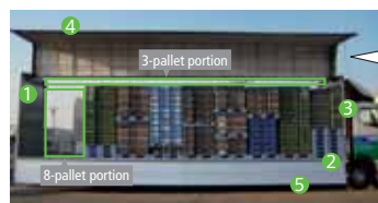
Enables an 11-pallet increase in loading capacity on a truck the same size as an 11t truck
