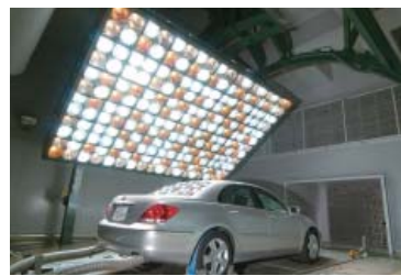
Environmental resistance testing (Reliability Center of DENSO Corporation)
