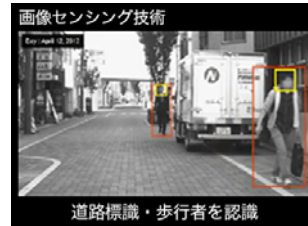
Detecting pedestrians through image sensing technology
