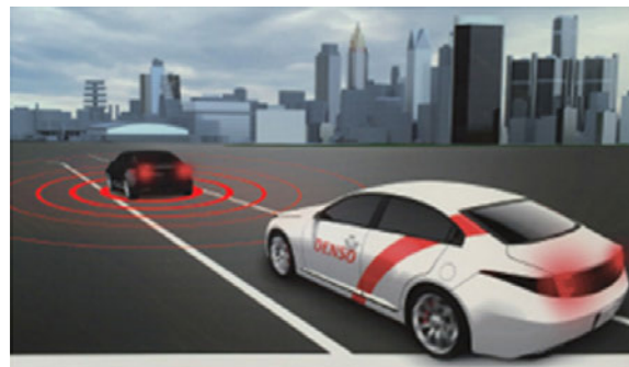
Safe stop by information of the lead vehicle The trailing vehicle safely stops in response to the sudden stop of the lead vehicle.
