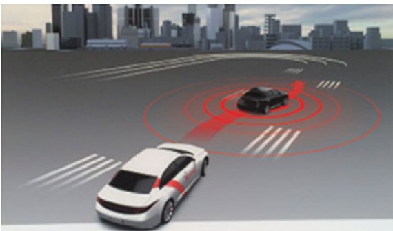
Following a lead vehicle The trailing vehicle uses positional information on the lead vehicle that is received by wireless to follow the lead vehicle at a safe distance.
