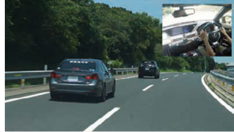
Public road test on Minamichita Road in Aichi Prefecture of single-lane automated driving (test vehicle is rear vehicle)
