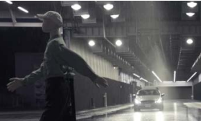
A natural environment test course that can replicate driving conditions at night or in the rain
