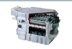
Double-sided cooling inverters (2007)
