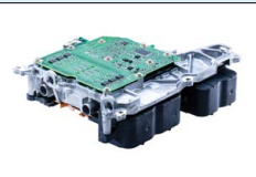
Inverters with SiC power semiconductors (2023)
