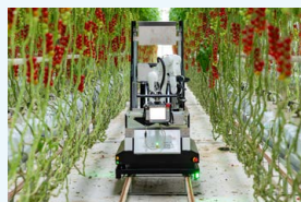
The fully automated cherry truss tomato harvesting robot Artemy ®
