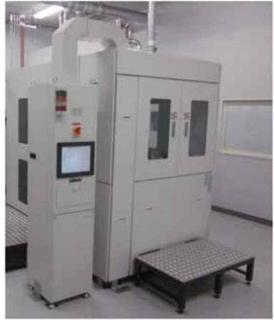
Fig. 21 High throughput Chemical Vapor Deposition
