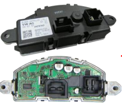
■ BPC (Blower Pulse Controller) to control HVAC motor
