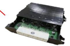
■ A/C ECU to control A/C Compressor.
