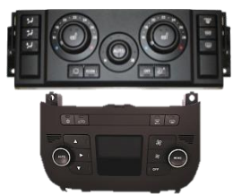
■ A/C Panel to control cabin temperature
