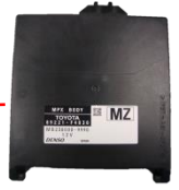
■ Main Body controls (Alarm, keys, comm, etc)
