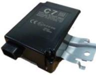
■ Smart ECU controls the centralized lock (keyless)
