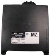
■ A/C ECU to control A/C Compressor.
