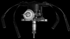
*DENSO's first Integrated Ignition Assembly (IIA)*
