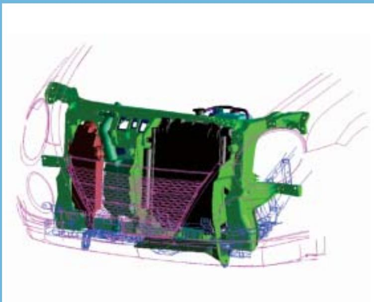
process—from the air inlets to the cylinder head ports. This leads to lower air intake noise levels, and improved engine performance. Integrating the engine ECU also removed the need for a separate ECU case and reduced the volume of wiring.
