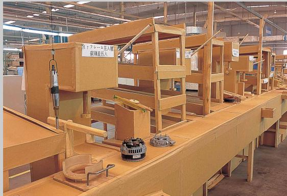
*Simulated production lines made of cardboard and wood.*
