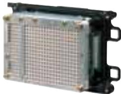
Millimeter-wave radar for pre-crash safety system
