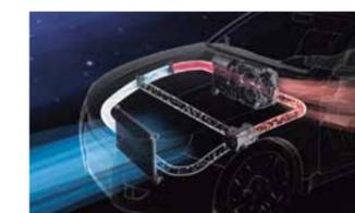
Heat pump system (rendered in-vehicle image)
