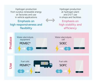
\* Proton exchange membrane electrolysis cell/Proton exchange membrane fuel cell. Joint development by the Toyota Group
