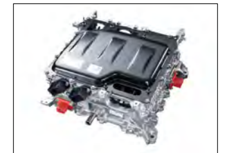
ESU (Electricity supply unit)
