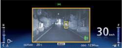
Night View System with Pedestrian Detection Function
