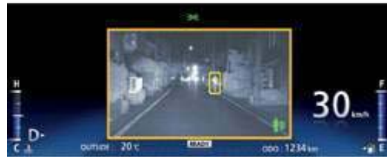
Night View System with Pedestrian Detection Function
