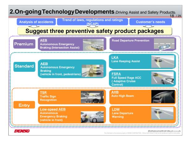
We will develop and propose three packages: Entry, Standard, and Premium, while taking into account of trends of laws, regulations and ratings (N–CAP) and customer needs in respective regions and will make these technologies into products in FY2016.
