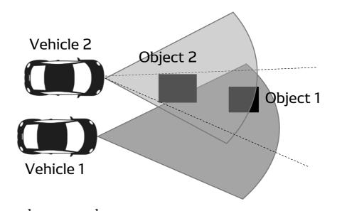
b) Occlusion based: Object 1 is more significant than Object 2 for vehicle 2 due to occlusion by Object 1
