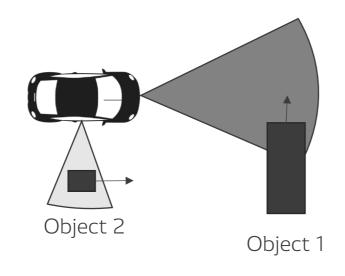
a) Kinematics based: Object 1 is more significant than Object 2 due to a potential collision path with the vehicle
