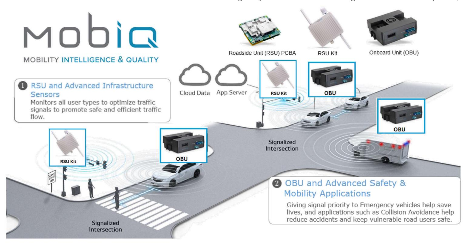
The MobiQ Onboard Unit supports advanced vehicle safety and mobility by connecting with Vehicle-to-Everything systems, Roadside Units (RSUs), and smart city infrastructure. Built on the Wireless Safety Unit's success, it offers a powerful development platform combining short- and long-range automotive communication. It enables vehicles, RSUs, and infrastructure to exchange critical data for safer and more efficient road use.
