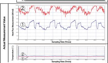
The amount of heat dissipation against CPU load fluctuation is visible
