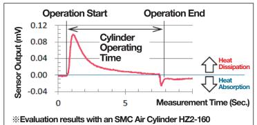
We could understand the operating condition of the air cylinder only by measuring on the pressure vessel surface
