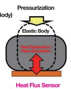
Heat dissipation / heat absorption occurred during deformation
