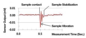
We could understand the sample static state by sticking a heat flux sensor to the stopper
