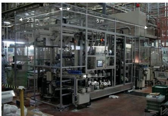
Fig. 8 Compact phosphate-lubrication equipment
