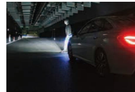
A nighttime pedestrian model used in our assessment of collision avoidance braking systems
