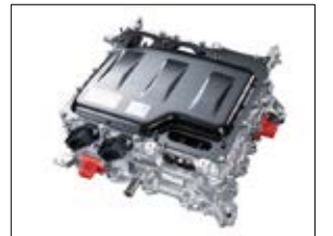
ESU (Electricity Supply Unit)
