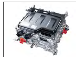
ESU (Electricity Supply Unit)
