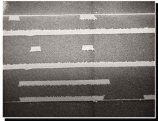
Fig.4 SEM of PCB for PEEK/PEI blends film: copper foil (18µm).
