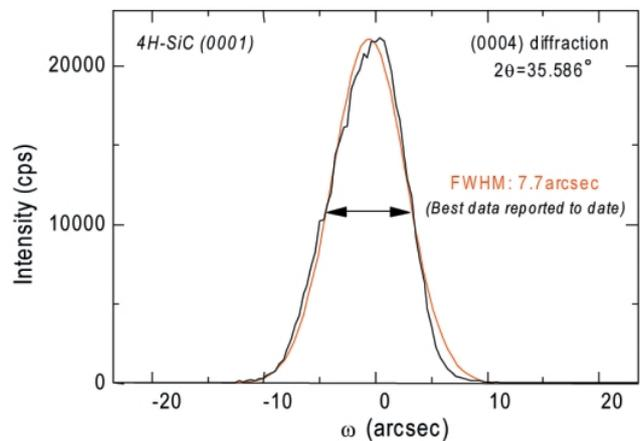
Fig. 1 HRXRD  $\omega$ -rocking curve of high quality of DENSO (HQ) wafers
