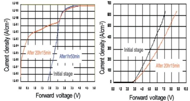
Fig. 4 (a) Forward characteristics degraded pn diode fabricated on reference wafer in (a) log, and (b) linear scale
