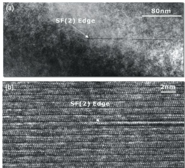
Fig. 6 Cross-sectional images of degraded pn diodes fabricated on 4H-SiC DENSO (STD) wafers (a) Low magnification, and (b) High magnification TEM images of stacking fault (SF2) edge in the drift epilayer region
