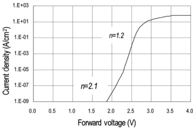
Fig. 2 Forward characteristics of pn junction diode fabricated on the DENSO HQ 4H-SiC wafers
