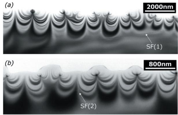
Fig. 5 Cross-sectional images of degraded pn diodes fabricated on DENSO (STD) wafers (a) Marked straight line corresponds to the stacking fault (SF1) nucleated near the implanted region/epilayer interface, and (b) Another stacking fault (SF2) terminated in the drift epilayer region
