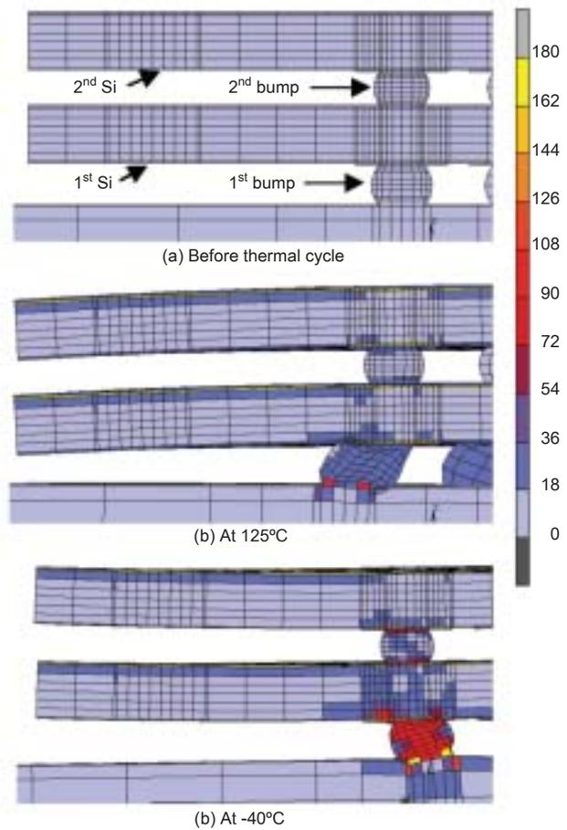
Fig. 5 Deformation and von Mises stress during thermal cycle, -40 to 125 °C (Deformation scale : 40)
