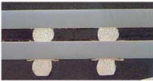
Fig. 4 Cross section of the connected 3D stacked package
