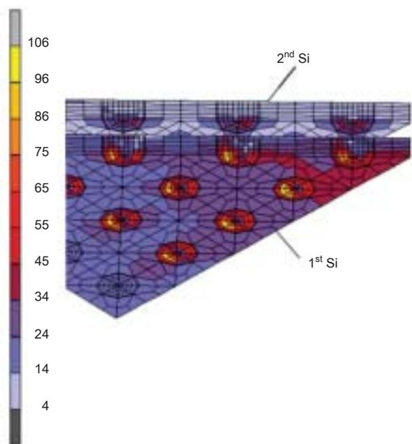
Fig. 7 Von Mises stress in Si chips at 125°C
