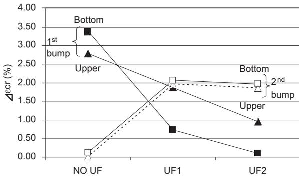
Fig. 13  $\Delta\epsilon_{cr}$  in solder bump at corner
