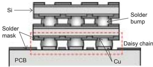
Fig. 1 3D-chip stacked package demonstrator
