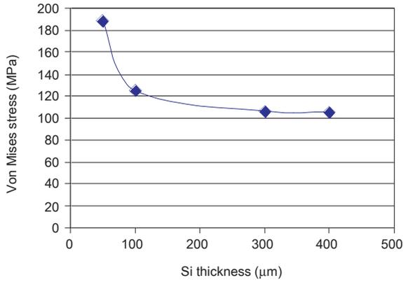
Fig. 9 Maximum von Mises stress in Si chips for different Si chip thickness
