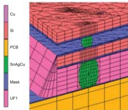
Fig. 12 FEM model of 3D chip stacked package with underfill
