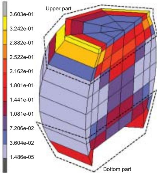
Fig. 6 Accumulated creep strain (-) in 1<sup>st</sup> bump (on PCB) in -40 to 125°C, 3cycles
