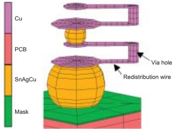
Fig. 10 FE model of 3D chip stacked package with Cu via hole and Cu redistribution path (Si and solder mask are eliminated.)
