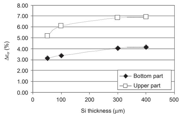
Fig. 8  $\Delta\epsilon_{cr}$  in 3D chip stacked package for different Si chip thickness
