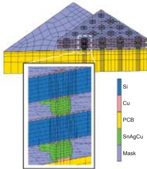
Fig. 2 FEM model for 3D chip stacked package
