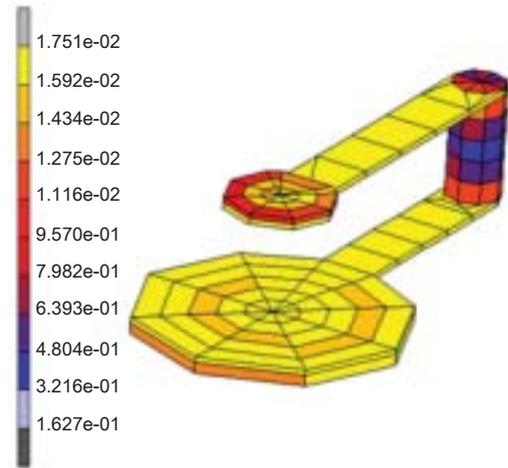
Fig. 11 Von Mises stress in Cu pad, re-distribution path and via hole at 125°C
