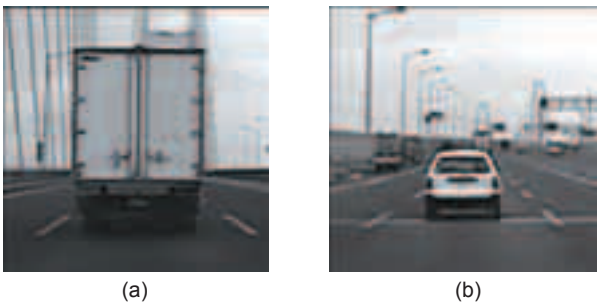
Fig. 3 Different types of target vehicle at same distance (a: Truck, b: Compact) and visibilities
