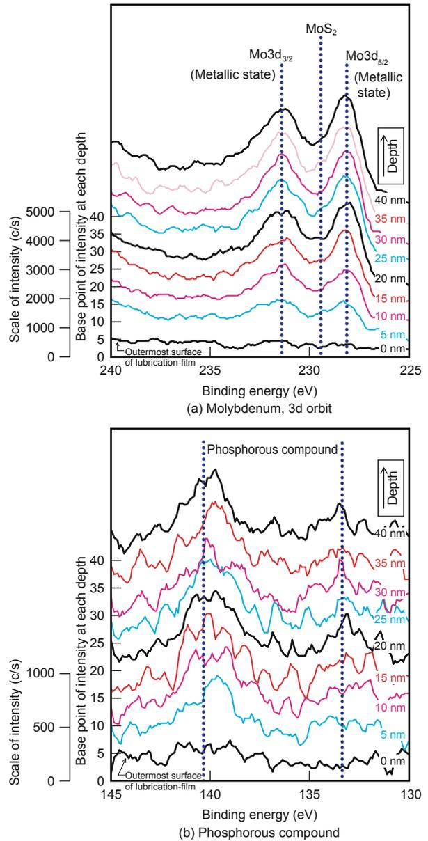
Fig. 21 Results of XPS of commutator sliding surface in depth-wise direction
