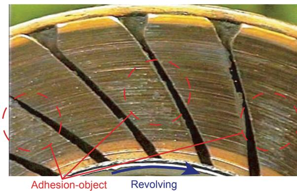
Fig. 11 Photo image of commutator sliding surface after starter start-stop endurance test with brush B
