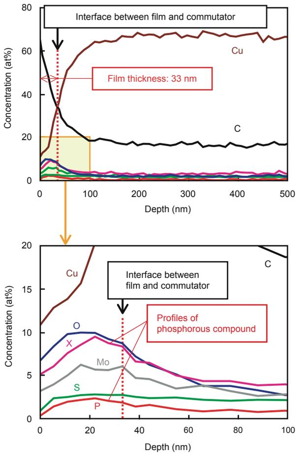
Fig. 20 Results of AES of commutator sliding surface in depth-wise direction
