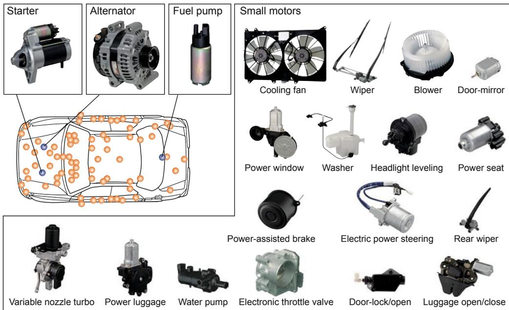
Fig. 1 Automotive motors and their installed positions
