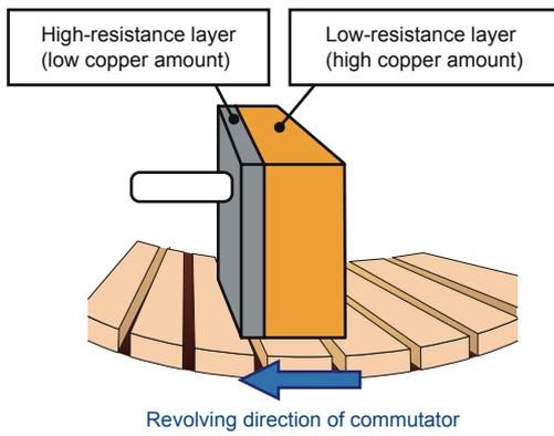
Fig. 4 Structure of two-layer brush
