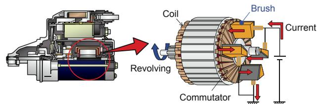
Fig. 3 Brushes and a commutator of a high-load starter
