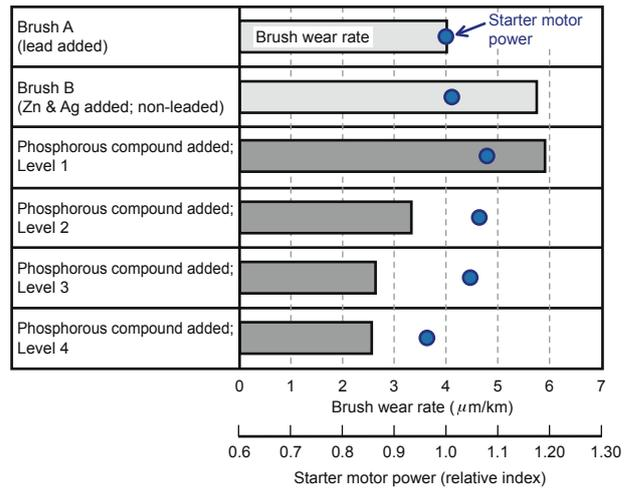
Fig. 16 Amounts of phosphorous compound and brush wear rates in starter motor start-stop endurance test/starter motor power
