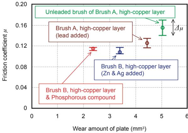
Fig. 15 Results of collar-plate friction and wear test
