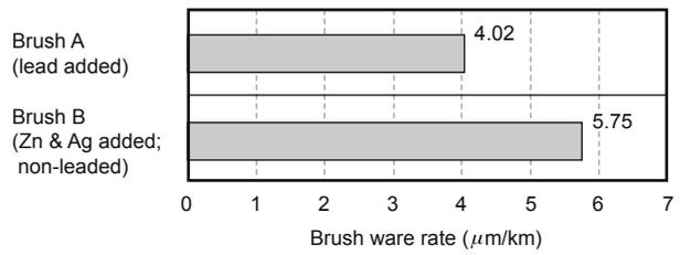
Fig. 5 Brush wear rate in starter start-stop-endurance test
