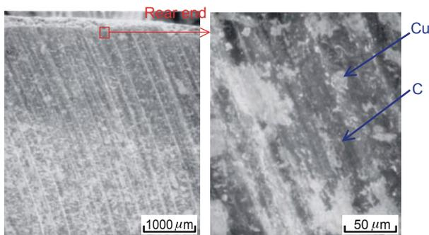
Fig. 19 SEM images of brush sliding surfaces after starter motor start-stop endurance test
