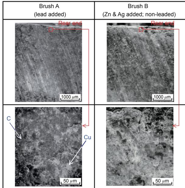
Fig. 12 SEM images of brush sliding surfaces after starter start-stop endurance test
