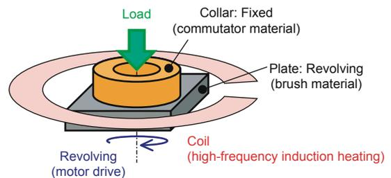
Fig. 14 Collar-plate friction and wear test apparatus
