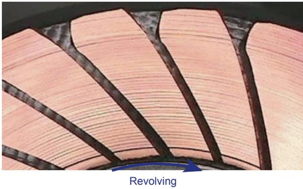
Fig. 9 Photo image of an unused commutator surface
