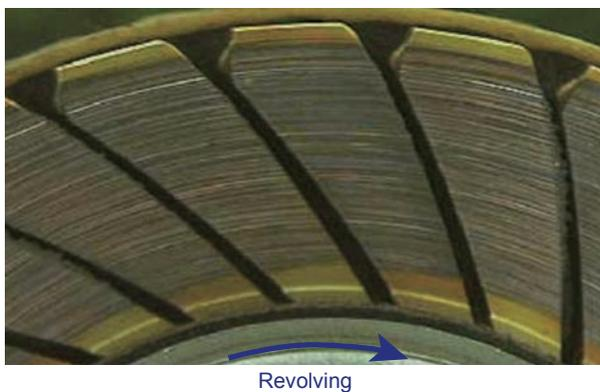
Fig. 18 Photo image of the commutator sliding surface after starter motor start-stop endurance test with developed brush
