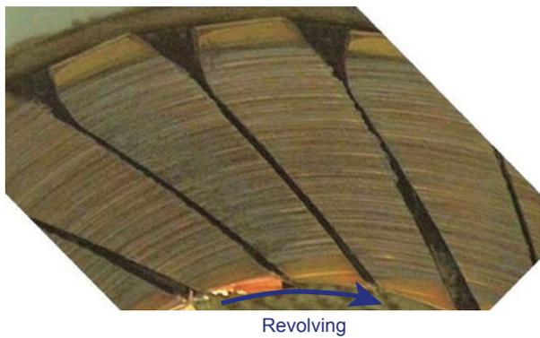
Fig. 10 Photo image of commutator sliding surface after starter start-stop endurance test with brush A
