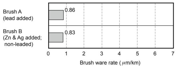
Fig. 7 Brush wear rates in sliding test
