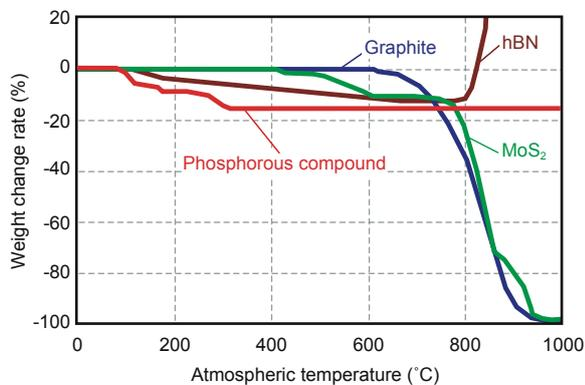
Fig. 13 Atmospheric temperature and weight change rates of solid lubricants (in air)
