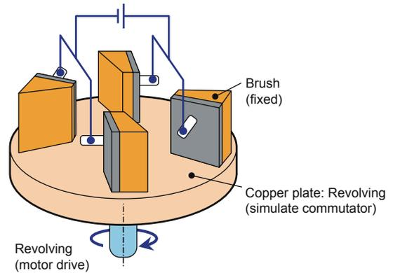
Fig. 6 Brush-copper plate sliding test apparatus
