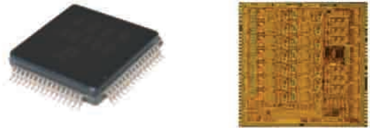
Fig. 12 Picture of the Integrated Circuit (left) and microchip contained within (right) that has been developed for the new Li-ion Battery Monitoring Unit
