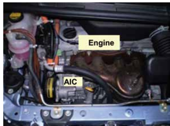
Fig. 10 AIC installed in engine compartment
