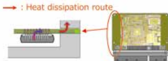
Fig. 12 Radiation structure from PCB to a case
