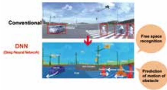
Fig. 26 DNN-IP Processing Result
