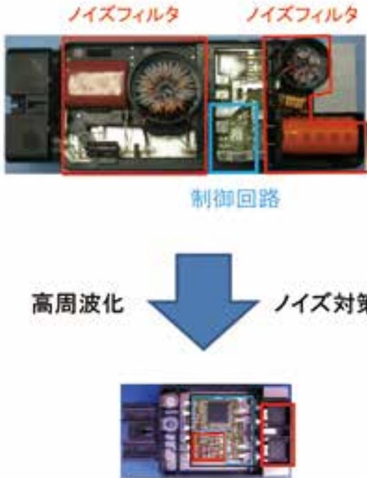
Fig. 6 Evolution of FPC (Fuel Pump Controller)
