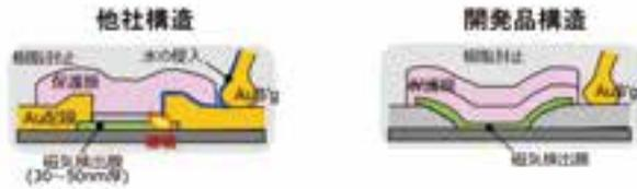
Fig. 11 Cross-sectional Structure of Thin-film Magnetic Sensor
