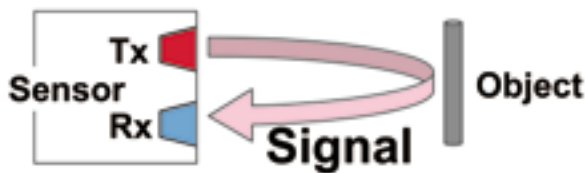
Fig. 1 Mechanism of the ranging sensor
