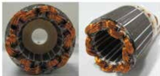
Fig. 14 Stator overview of a prototype motor
