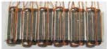
(b) Stator core after inserting formed distributed windings
