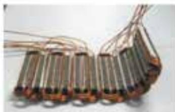
(c) Bent stator core with windings
