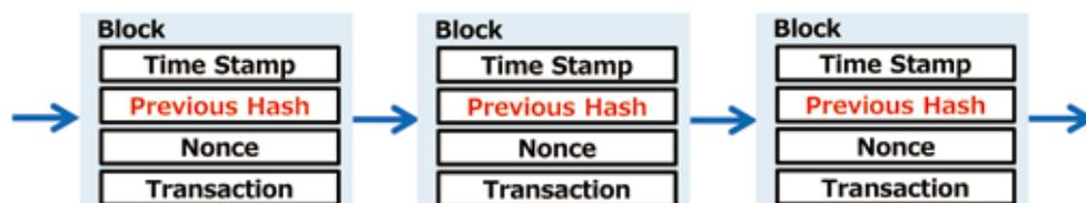
Fig. 2 Blockchain connected by Hash value
