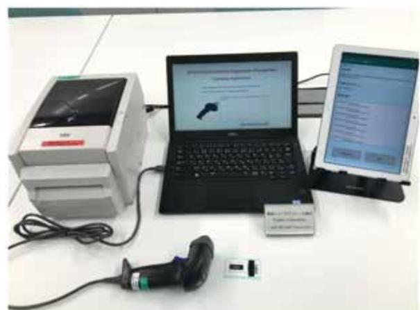
Fig. 11 Total system of traceability using blockchain and secure QR code
