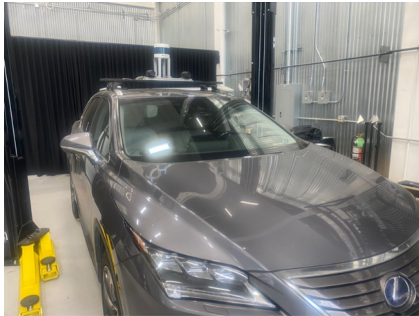
Figure 1: Lexus RX450hL Equipped with a Velodyne VLS-128
