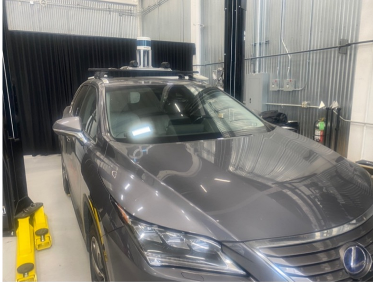
Fig. 2: Lexus RX450hL Equipped with a Velodyne VLS-128
