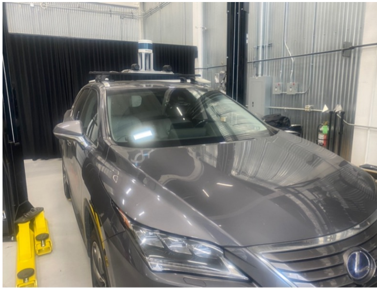
Fig. 2: Lexus RX450hL Equipped with a Velodyne VLS-128
