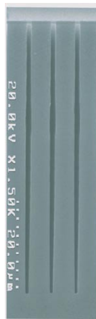
Fig.12 Etching example (Trench depth: 62.6 μm, Trench width: 1.05 μm, Aspect ratio: 60)
