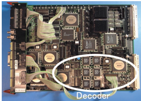
Fig. 7 Photograph of demodulation hardware with Predicative Decoder
