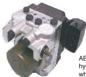
ABS actuator controls the brake hydraulic pressure for each wheel cylinder.
