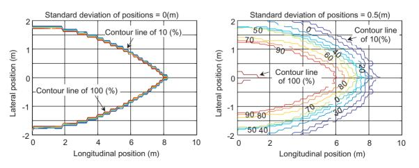
Fig. 10 Examples of collision probability map
