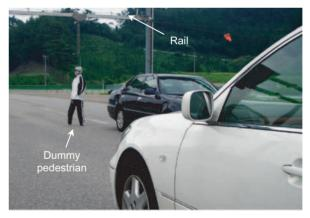
Fig. 4 An example of test scenario and facility for pedestrian sensing test
