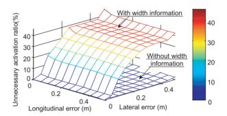
Fig. 12 Unnecessary activation ratio on 0.1m gap passing
