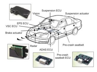
Fig. 2 An example of ADAS configuration
