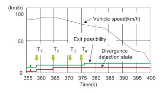
Fig. 7 An example of divergence detection result
