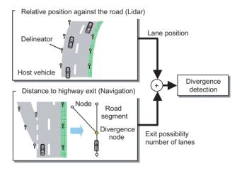
Fig. 6 Outline of divergence detection algorithm
