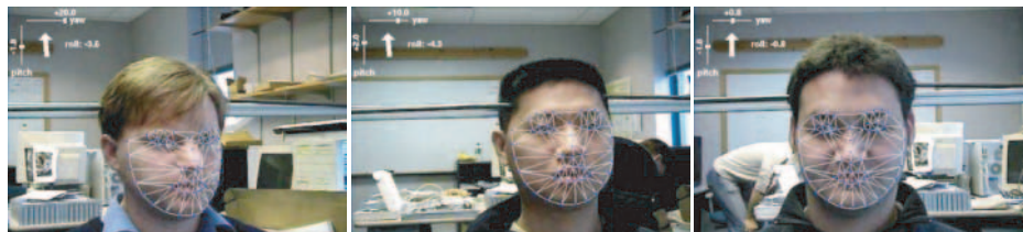
(a) Ground truth (20, 0, 0) Result value (20, -1.8, -3.6) (b) Ground truth (10, 0, 0) Result value (10, 2.0, -4.3) (c) Ground truth (0, 0, 0) Result value (0.8, -1.8, -0.8)
