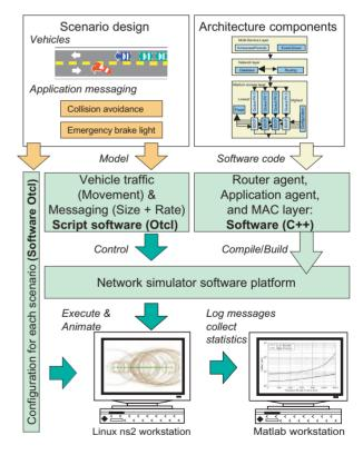
Fig. 8 Work required for simulation
