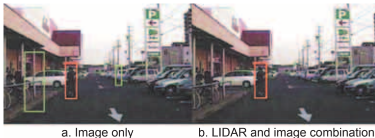
Fig. 5 Illustration of the reduction of false positives due to the use of LIDAR
